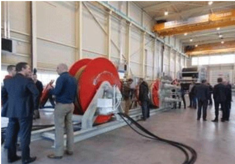
**IHC Winches has presented its 50 ton fiber rope traction winch, known as IDsis, to the Dutch and Belgian offshore markets.**
